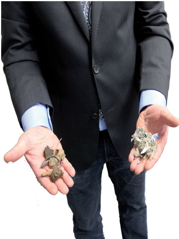
3. Thomas Jennewein shows two extremes of AF: On the left a very light AF (mixture of wood chips and rubber) which might be used in a calciner; on the right an AF (RDF mixture of plastic, paper and shredded carpet) which might be used for a main burner
