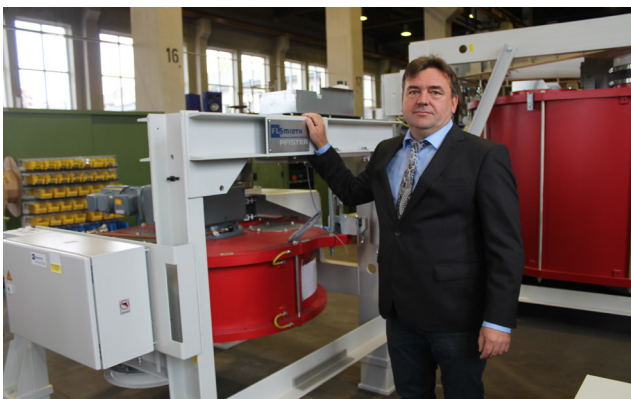
1. From small to huge: Thomas Jennewein shows Pfister rotor weighfeeders for alternative fuels set up for different, individual demands
