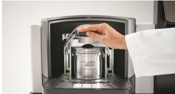
Easy closing of the clamp, automatic locking via ServoLock
