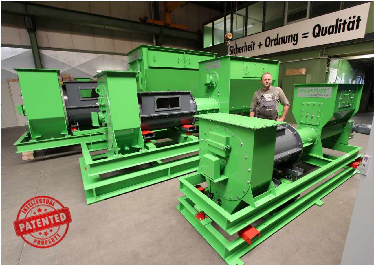
Fig 7: The novel patented ODM WeighTUBE® tubular weighing system
