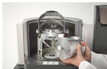
Safely guided insertion of the grinding bowl
