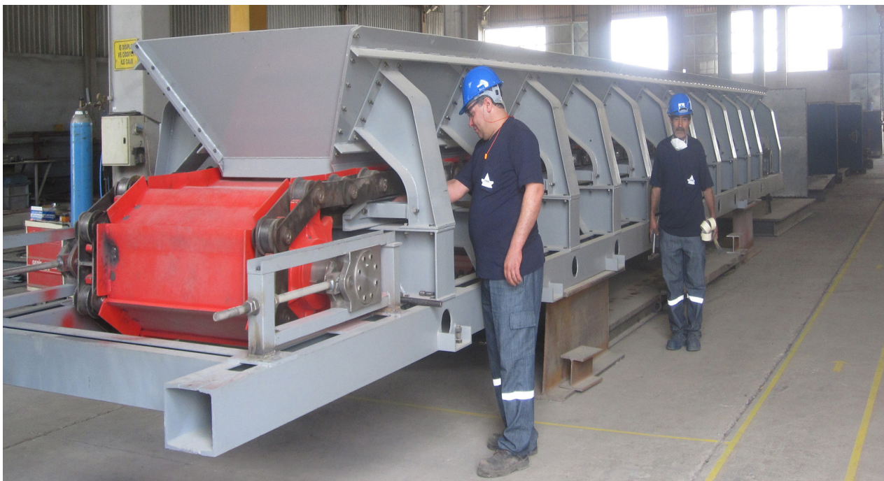
Fig. No. 09 - Apron Feeders
