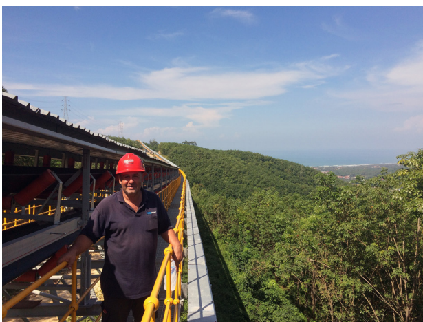
Figure 6: Achmed Ammoura, chief erector in the BEUMER Group, at the belt conveyor with horizontal curves
