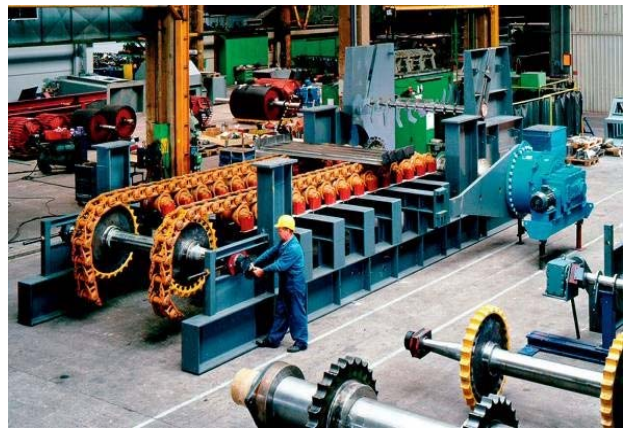
AUMUND Type BPB-SF during works assembly
