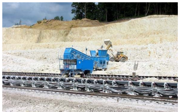
Mobile Feed Point to Field Conveyor
