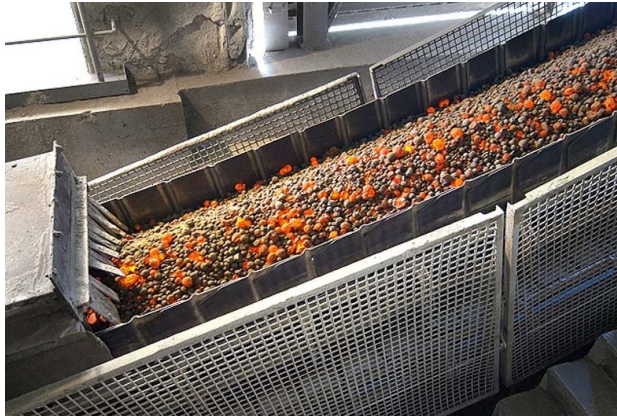
AUMUND Pan Conveyor (type KZB) handling hot material
