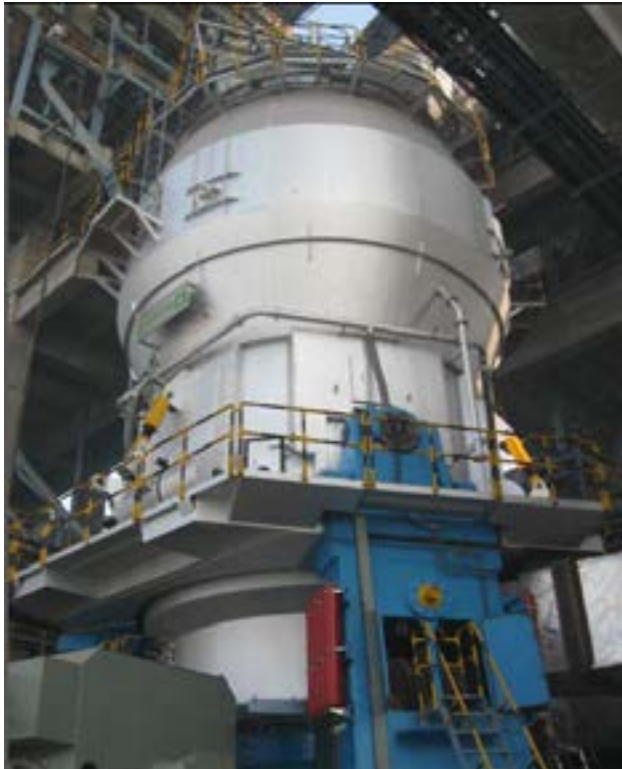
Similar mill type LM 56.3 + 3 installed in Dadri, India
