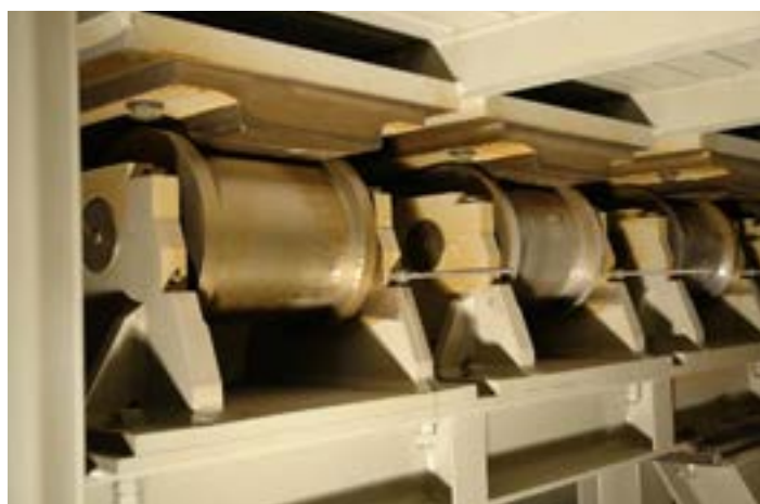
Fig. 6: Lane support inside chamber with heavy duty roller.
