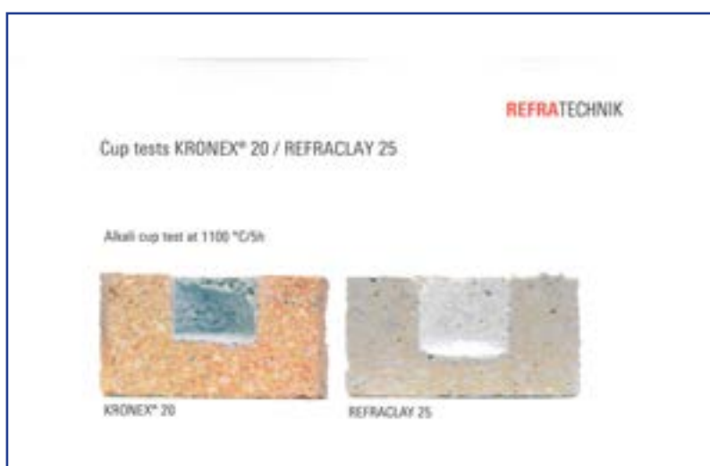
Figure 5: Cup corrosion tests
