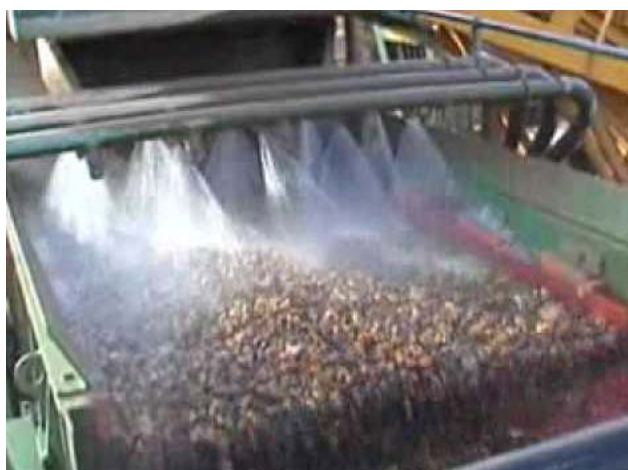
Fig. 5: Raw material washing nozzles equipment
