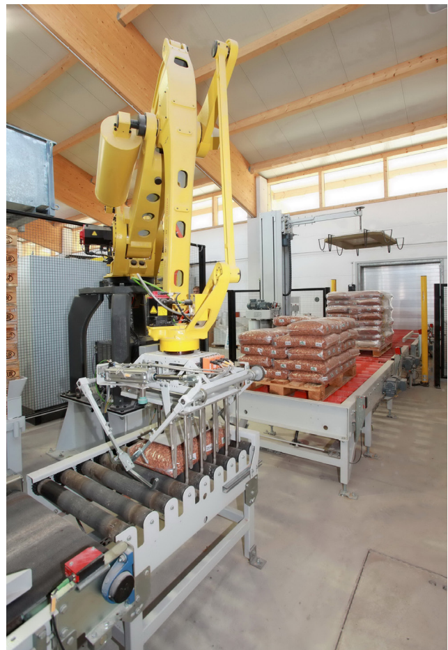
Fig. 4: The BEUMER robotpac series palletises and depalletises a wide range of packages using specially developed gripping systems.
