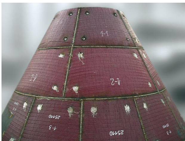
Figure 7 KALMETALL-W 100 hard overlay welded plates protect the vertical mill zones that are exposed to sliding and impact wear.
