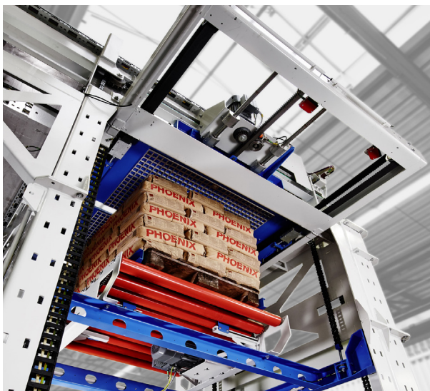
Fig. 2: The BEUMER paletpac forms exact, stable and thus space-saving bag stacks.
