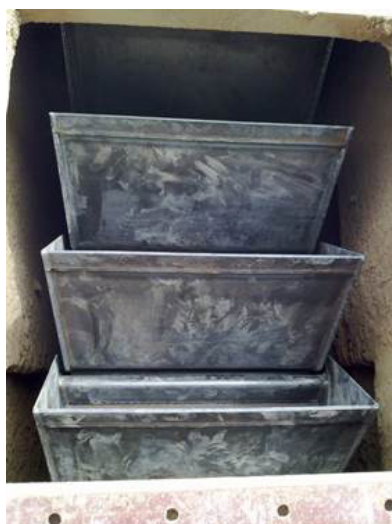
Fig. 1) AUMUND Belt Bucket Elevator type BWG-GK for coarse grain: The narrow, overlapping bucket configuration permits the belt to disappear entirely behind the buckets. No coarse material will be thrown behind the backs of the buckets, even after stoppage
