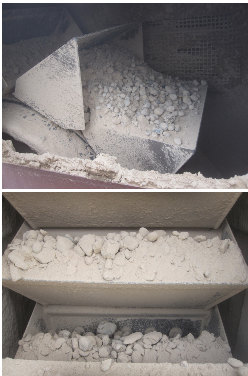
Fig. 1) AUMUND Belt Bucket Elevator type BWG-GK for coarse grain: The narrow, overlapping bucket configuration permits the belt to disappear entirely behind the buckets. No coarse material will be thrown behind the backs of the buckets, even after stoppage
