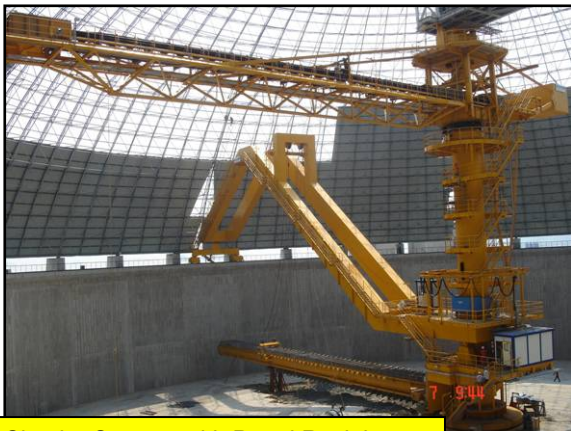
Circular Storage with Portal Reclaimer
