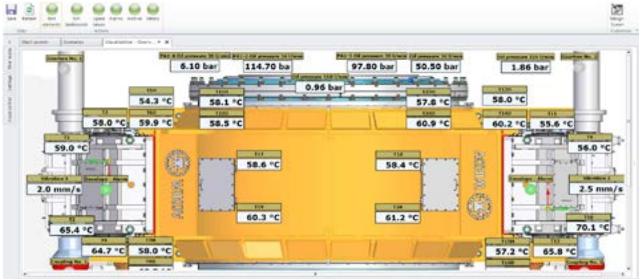
A screen-shot from WiGuard, which allows Wikov's engineers to see a raft of key parameters remotely.
