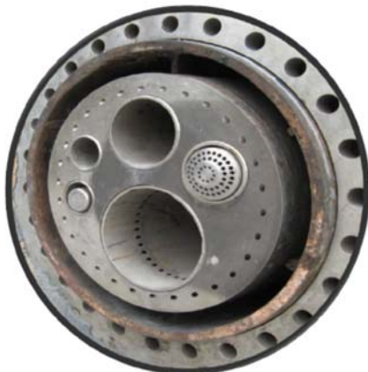
Turbu-Jet burner with large lofting air channel for solid alternate fuels
