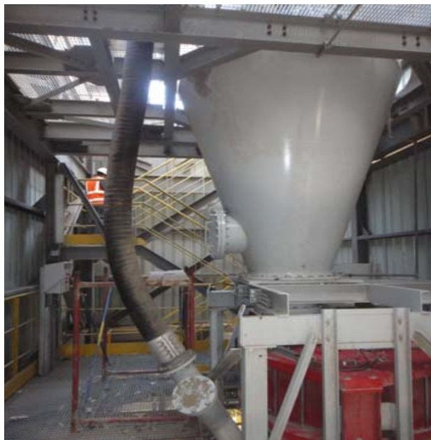
Pic 5: Adel Ezzat, Alternative Fuel Manager at Arabian Cement shows the FLSmidth Pfister installation for dosing alternative fuels at the cement plant in Ramliya, Egypt
