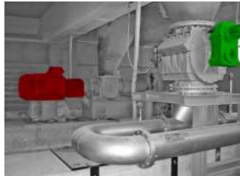
Figure 9: Comparison motor size screw pump vs. rotary valve
