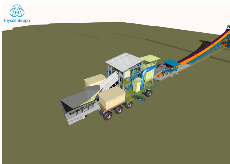
Primary Mobile Crusher for Limestone
