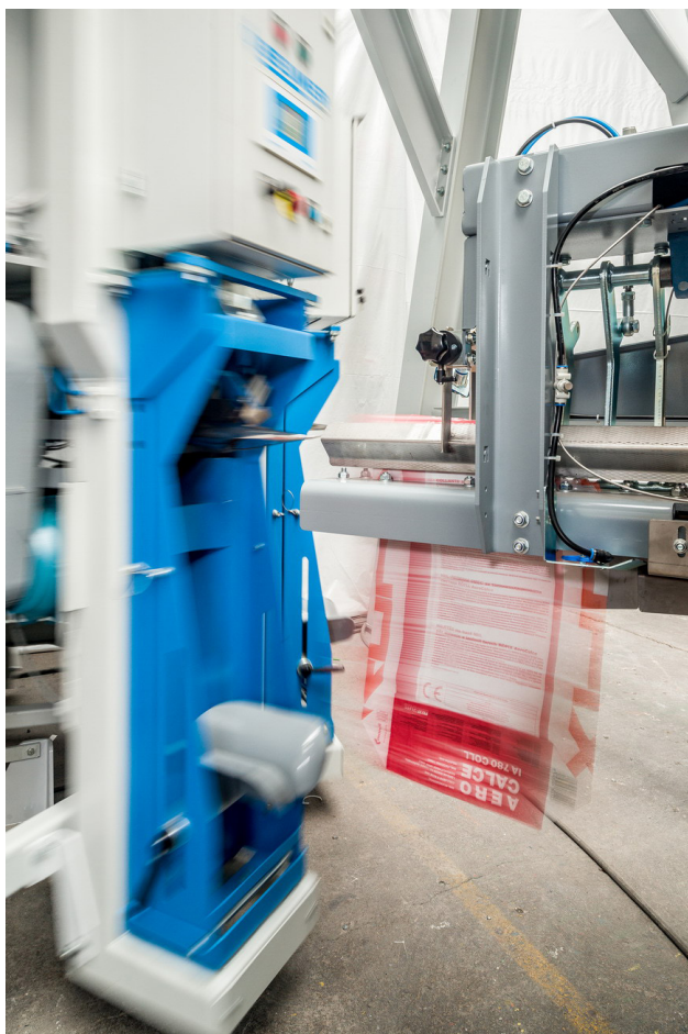
Picture 1: The bag placer applies the valve bag with precision on one of the filling spouts of the BEUMER fillpac R
