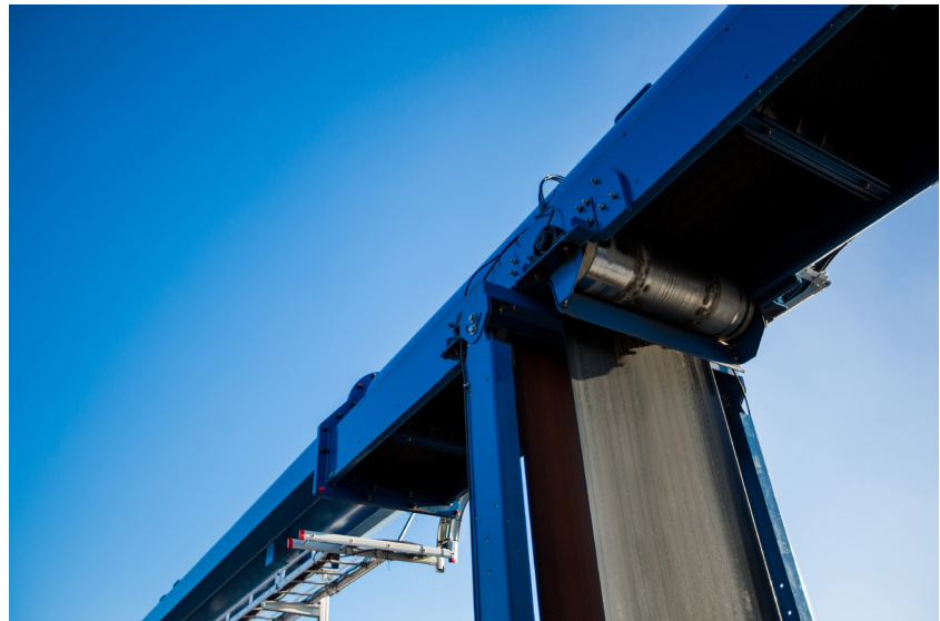
Picture 1: Additional scrapers mean fewer maintenance costs, fewer downtimes and less material carry-over.
