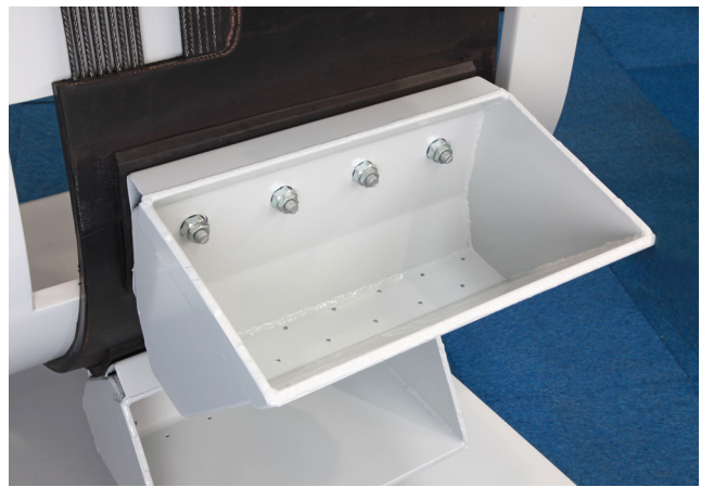
Photo 2: In the scope of the modernisation at Lafarge, the belt bucket elevator has been upgraded with the BEUMER heavy-duty technology. The new bucket shape ensures smoother running and less generation of noise.
