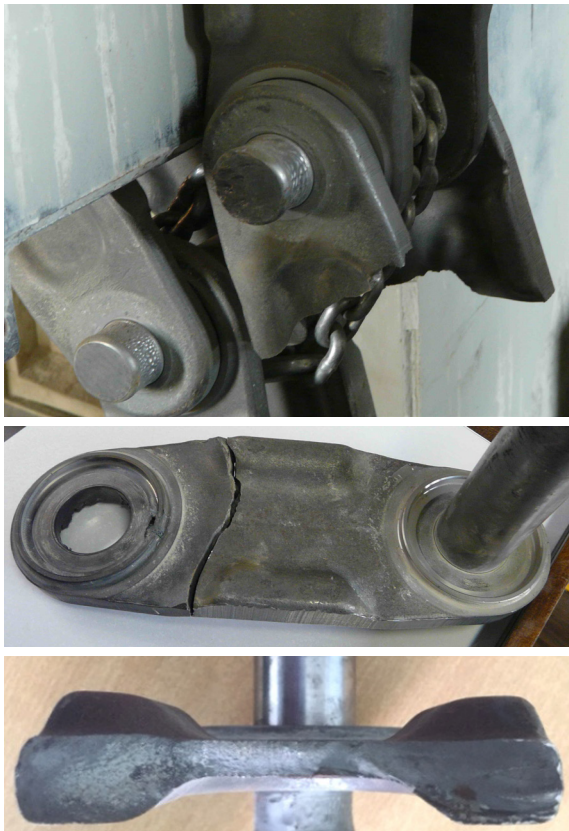
Fig. 6 Exemplary photographic images of broken outer links of bucket elevator central chains with old design
