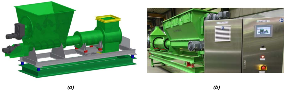
Figure 4- ODM-WeighTUBE® - High precision tubular weigh feeder: (a) - 3D Model, (b) - Real machine (back) and control system (front)
