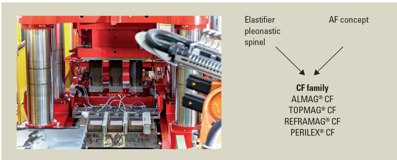
Figure 6: Pressing of innovative basic bricks (CF concept)
