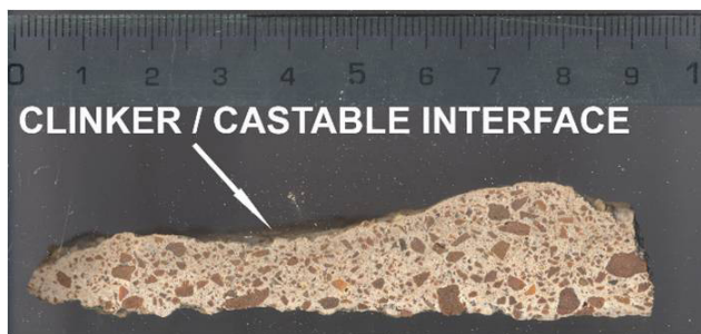
Fig. 7: Cross section of Magnesia-Spinel castable after the service.
