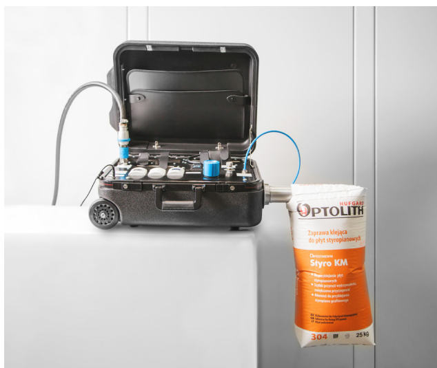
Picture 1: The BEUMER bag tester enables users to exactly determine the venting capacity of any type of valve bag.
