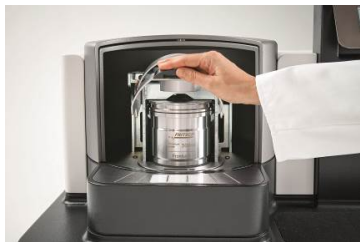
Easy closing of the clamp, automatic locking via ServoLock
