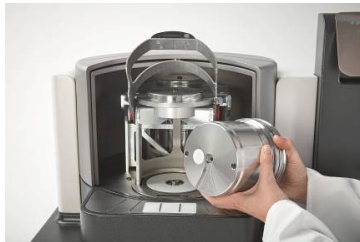
Safely guided insertion of the grinding bowl
