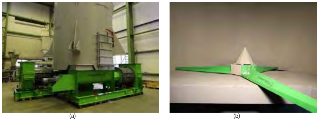
Figure 10- ODM-MultiTUBE arrangement: (a) shared buffer and two dosing lines; (b) ODM-RotoEX silo extraction system
