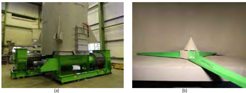
Figure 10- ODM-MultiTUBE arrangement: (a) shared buffer and two dosing lines; (b) ODM-RotoEX silo extraction system
