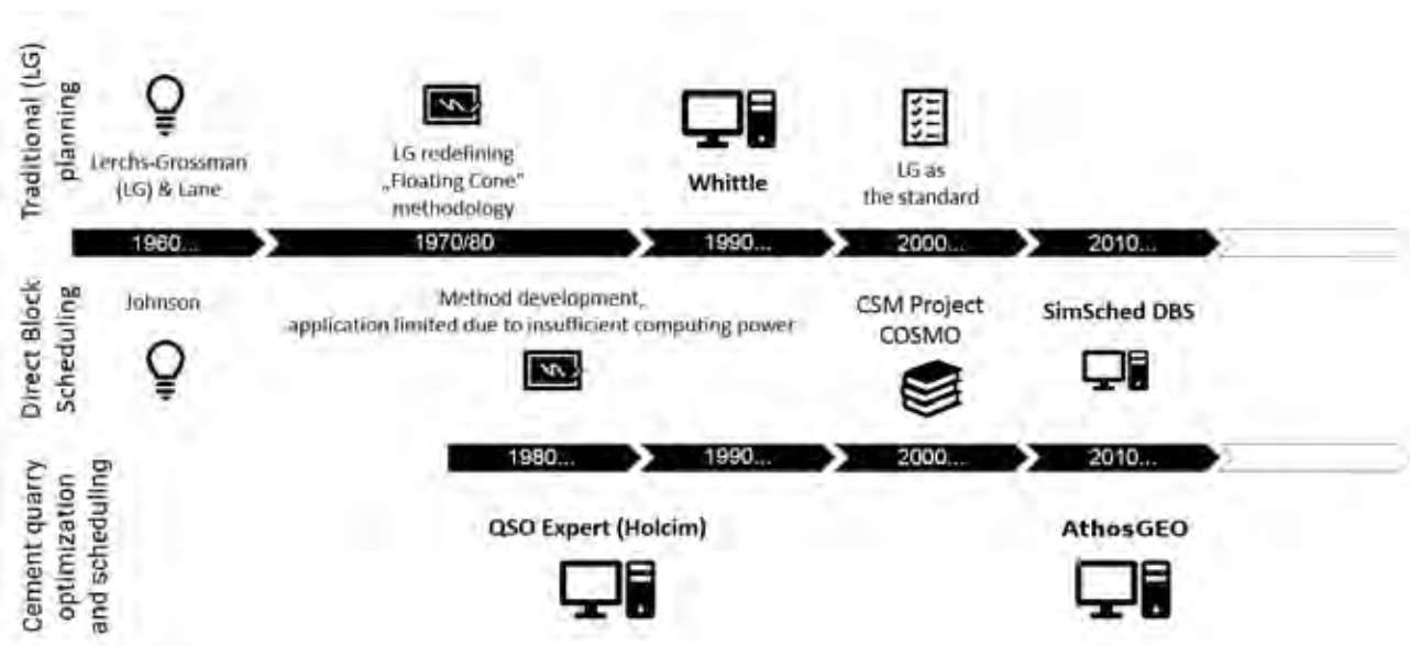
Figure 5 Development of computerized mines planning concepts. The methods going back to Lerchs-Grossman (LH), like the Whittle software, are nowadays dominating the resources and reserves estimation in metal and other major mining industries. Direct Block Scheduling (DBS) methods are solving the same optimization problems in a stricter way, but they require computing power (like 64-bit hardware) that is only recently available. However, mining for cement faces different challenges and the market of available software is much more restricted.
