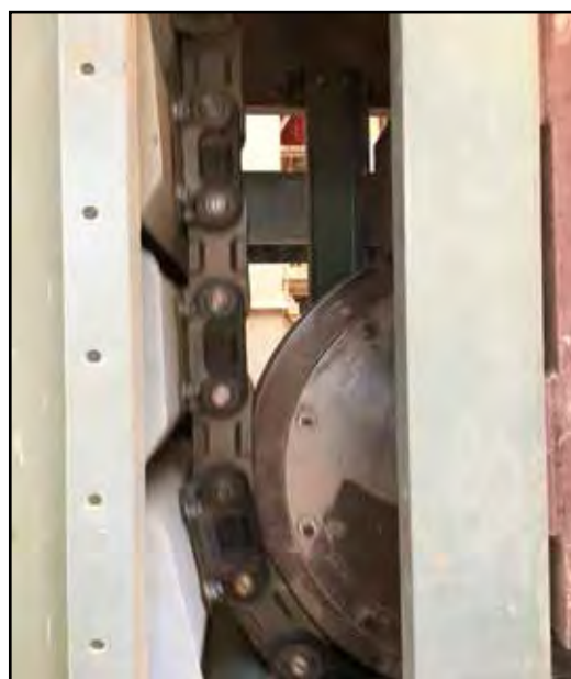
Fig. 4: The Heko central chain is extremely powerful, offering a breaking load of 1450 kN.
