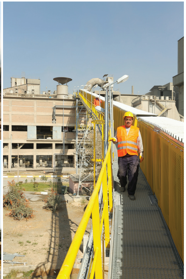
Picture 5: The second line transports fuels to the main burner.
