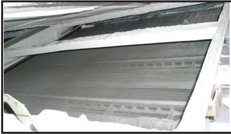
Figure 1: Screening surface after three month of continuous operation with a magnetic drive.
