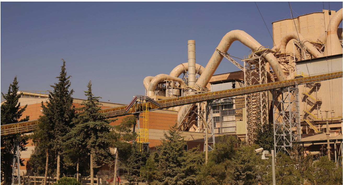
Picture 1: BEUMER Group supplied and installed a single-source solution based on the innovative Pipe Conveyor technology.
