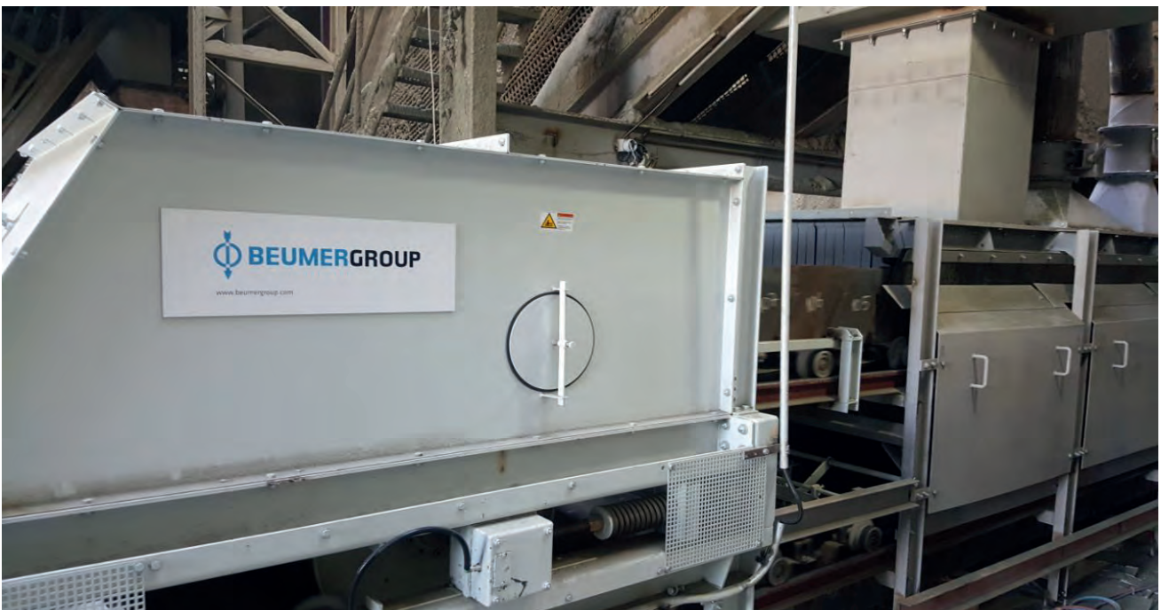
Photo 2: The slim and weight-reduced design of the GSZF reduces the costs for steel structure and freight. The operator was able reduce costs considerably.
