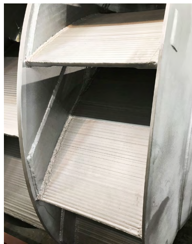
Pic 2: New, state-of-the-art wear protection helps to increase the lifetime and performance range of the fans.
