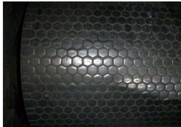
Hexadur® surface after 33600 hours of operation Expected Lifetime of wear surface more than 100000 hours of operation.
