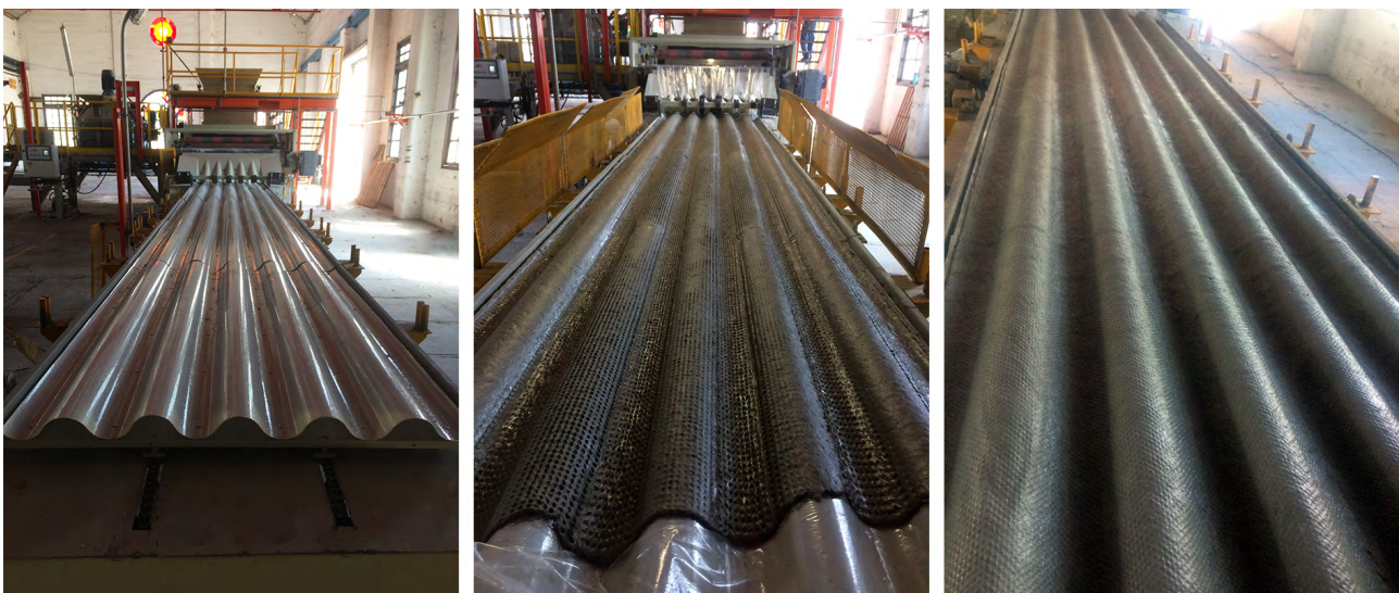
Figure 3. Continuous sheet produced using the VIDMAR system before longitudinal cutting
