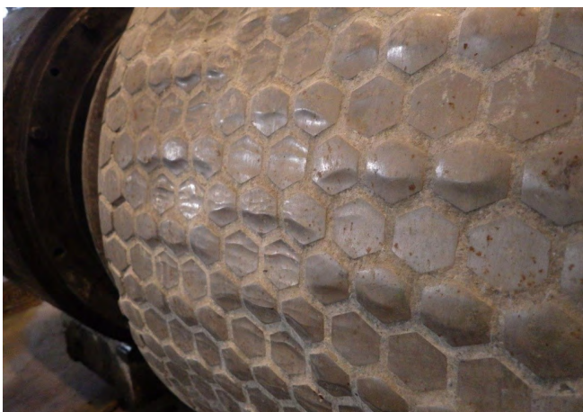
Hexadur® surface after 76000 hours of operation
