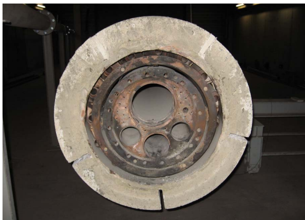
Kiln main burner for using four different fuels simultaneously.
