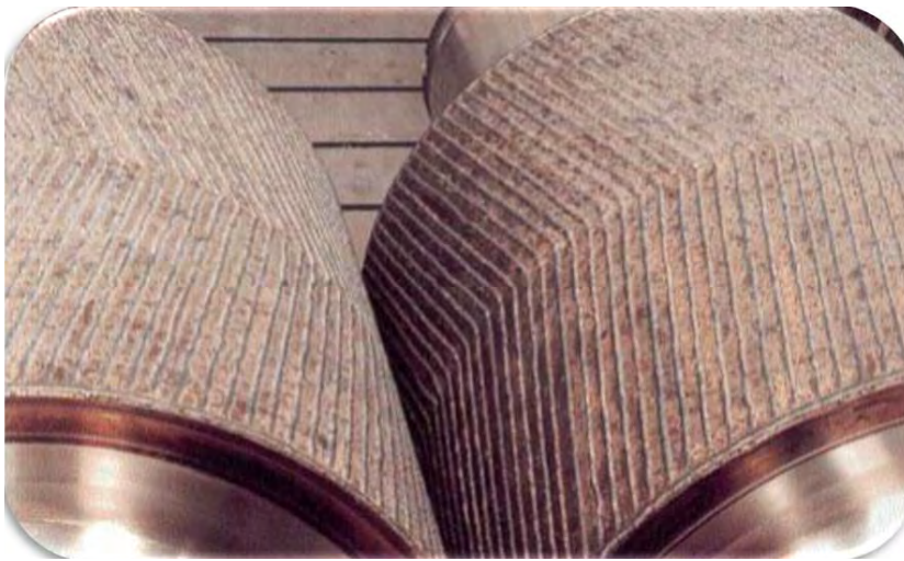
New hard faced rollers
