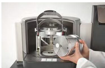
Safely guided insertion of the grinding bowl
