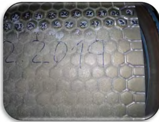
Hexadur® surface after 38600 hours of operation. Expected Lifetime of wear surface .more than 100000 hours of operation
