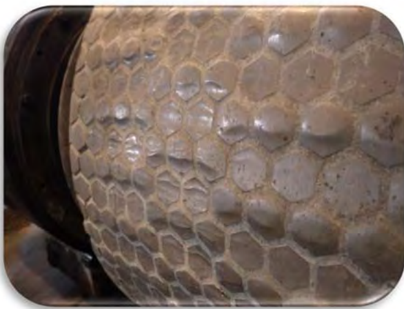
Hexadur® surface after 76000 hours of operation
