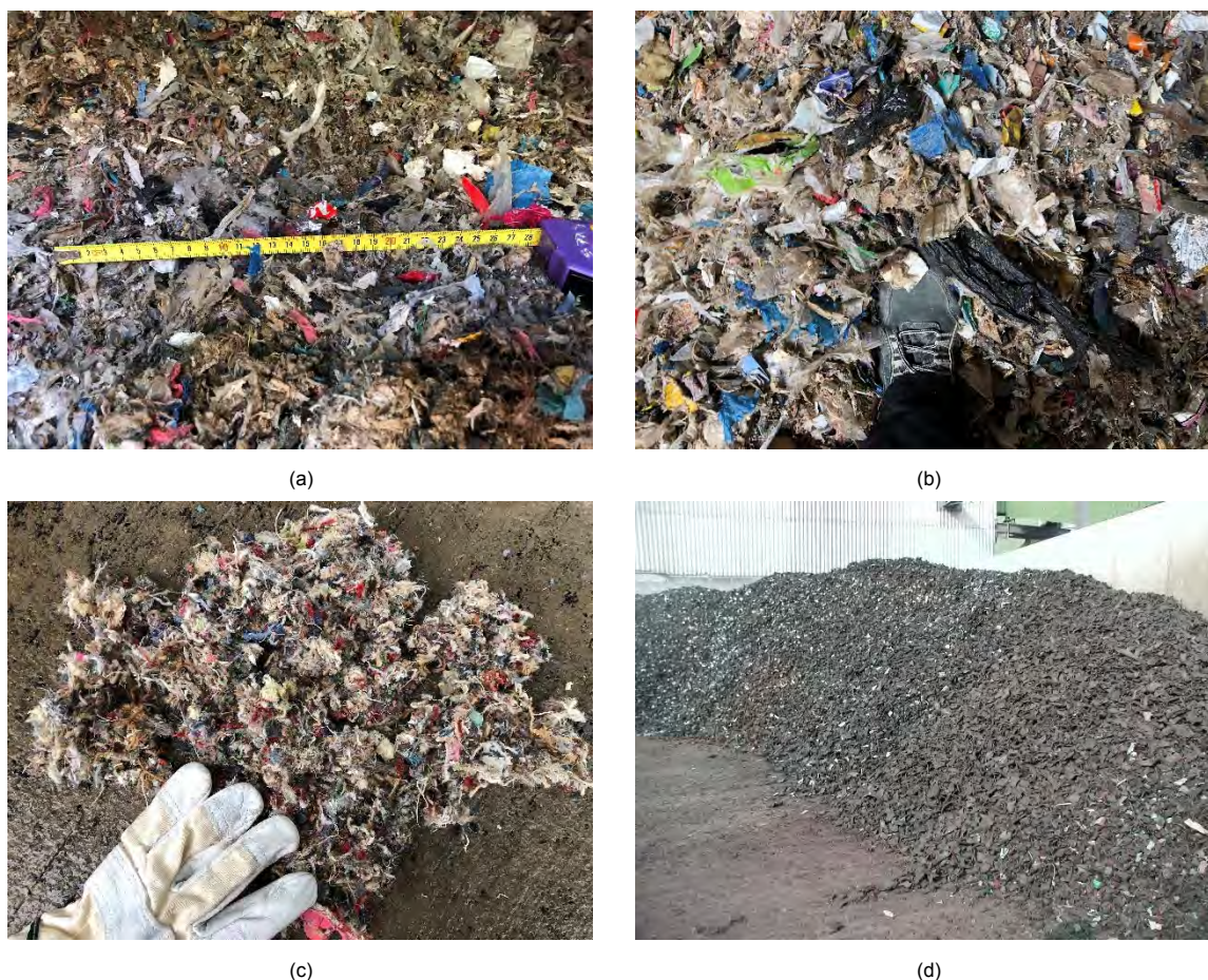
Figure 4 - Different types of fuels: (a) – Typical fine fuel (RDF) for main burner; (b) – Coarse fuel (RDF) for calciner feeding; (c) – Example for agglomerated fuel (here: carpet fluff); (d) – Coarse tire chips
