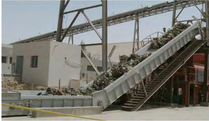
Figure 7 - ODM_GFK surface feeder for the reception and transport of coarse alternative fuels
