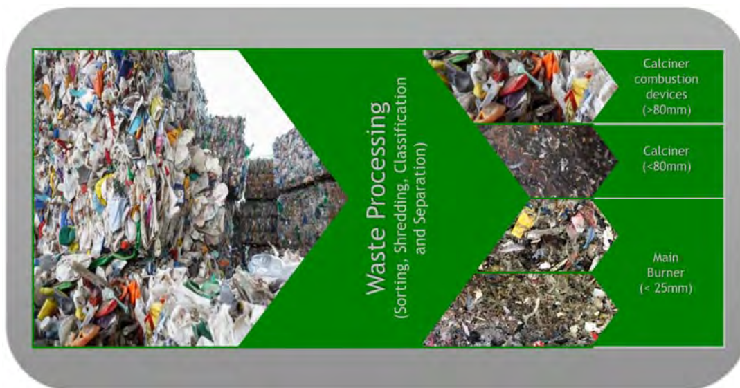
Figure 5 - Fuel preparation and processing and associated thermal processes
