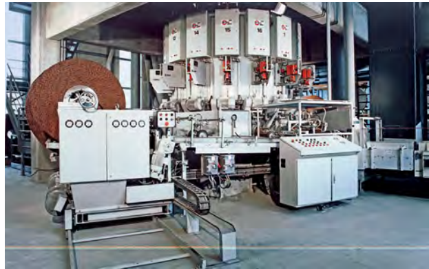
ROTO-PACKER® using the turbine filling system and an automatic bag applicator
