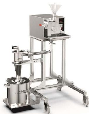
Universal Cutting Mill PULVERISETTE 19 with new FRITSCH high-performance Cyclone separator
