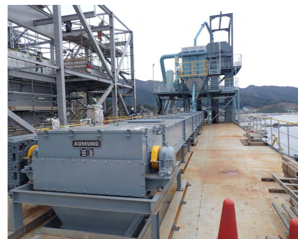
AUMUND Drag Chain Conveyor type TKF
