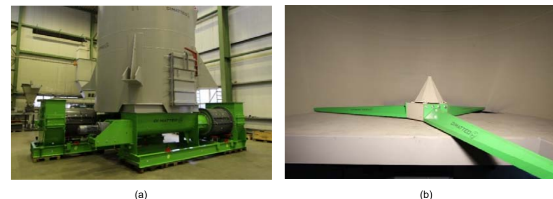
Figure 5- Combination of storage and dosing units; (a) – Two ODM-WeighTUBE ® directly mounted below a circular silo; (b) – ODM-RotoEX silo discharge system for a robust homogenous discharge
