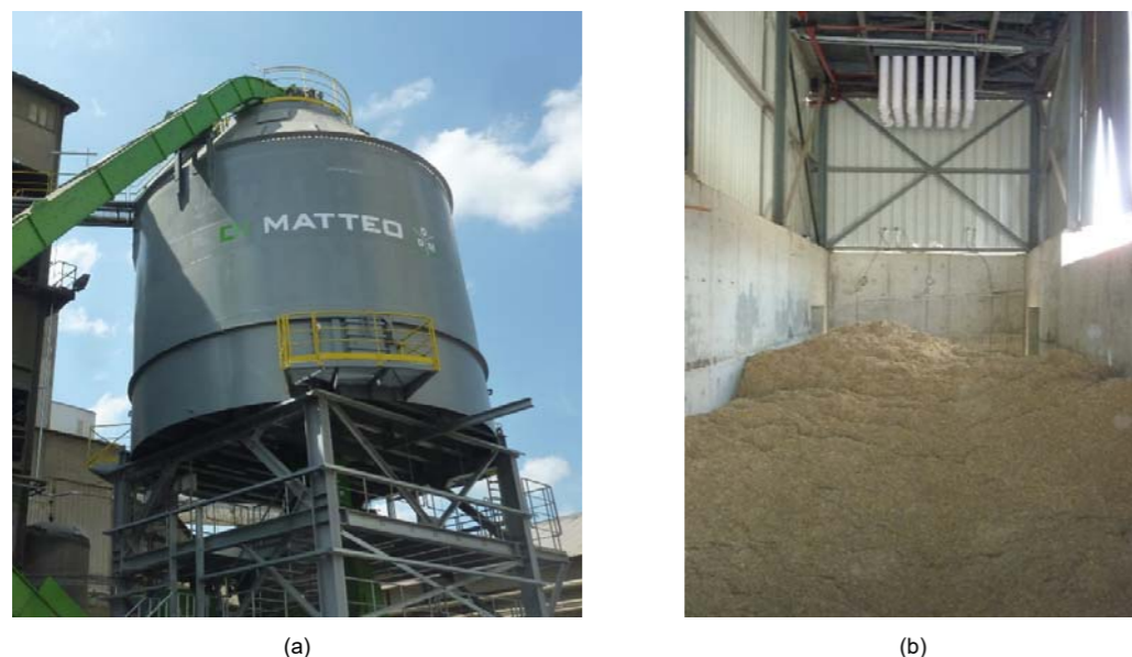
Figure 4- Typical shapes of storages: (a) – Classical circular shaped silo; (b) – Rectangular storage hall
