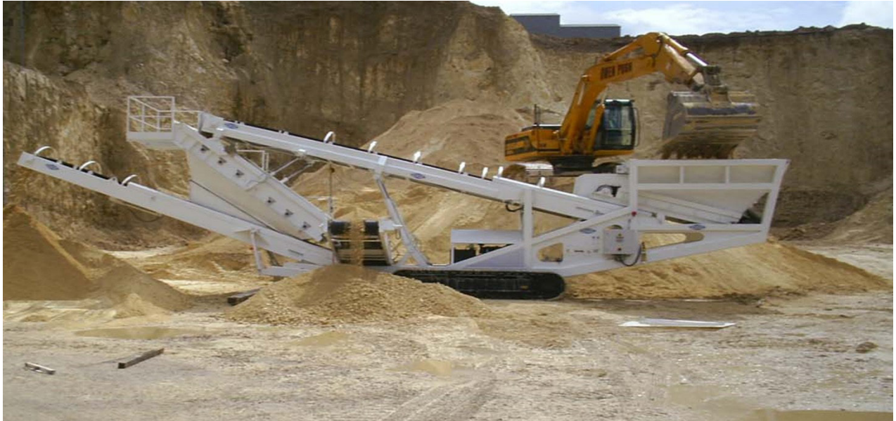
Figure 3: Mobile sand classification with the RHEWUM Liberty Screen (Source: RHEWUM)
