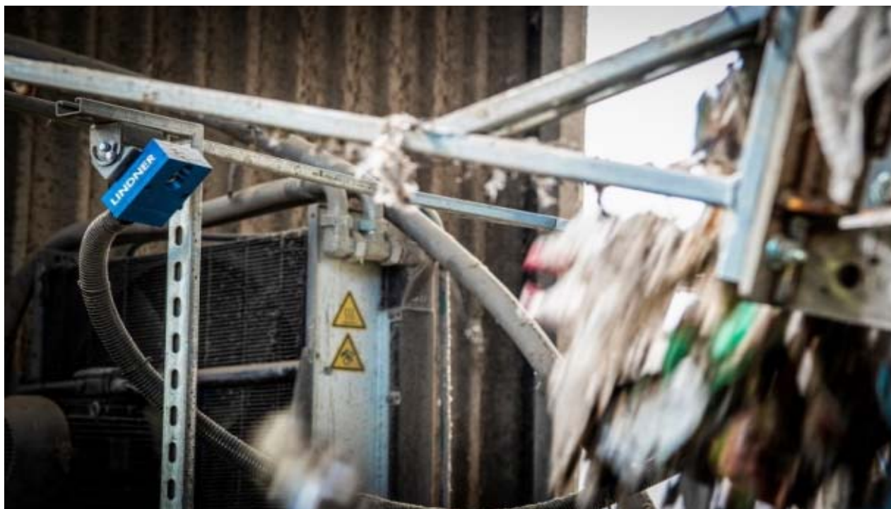
Fig. 4: Lindner's Fire Prevention System (FPS) sensor instantly detects overheated particles after the first shredding unit
