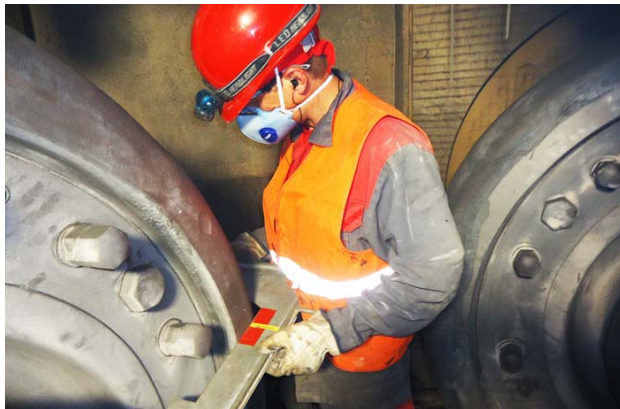
An application specialist of vertical mill is check wear profile of mill roller.
