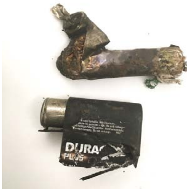
Fig. 1: Batteries damaged during mechanical processing, when converting waste into SRF, pose an enormous fire hazard
