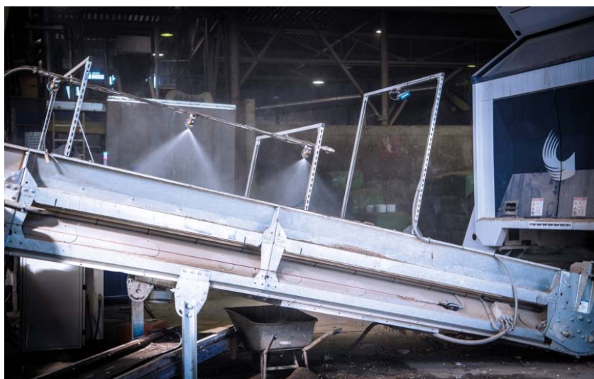
Fig. 3: Cooling after the first sensor was triggered
