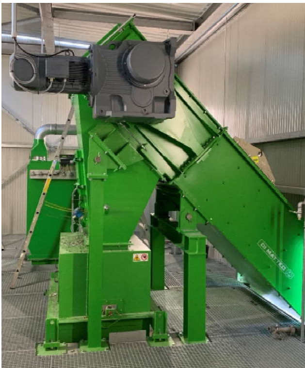
(a) (b) Figure 6 - ODM-MAS magnetic separator – (a): machine; (b): typical rejects
