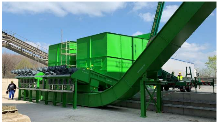
Figure 4 – ODM-ScrewDOS ® screw bottoms and ODM-TKF drag chain conveyor
