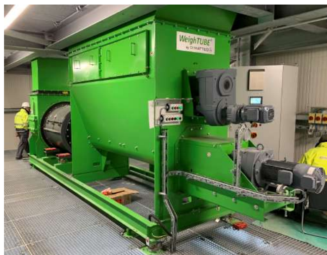
Figure 7- ODM-WeighTUBE ® gravimetric dosing system incl. ODM-GravitAS control system
