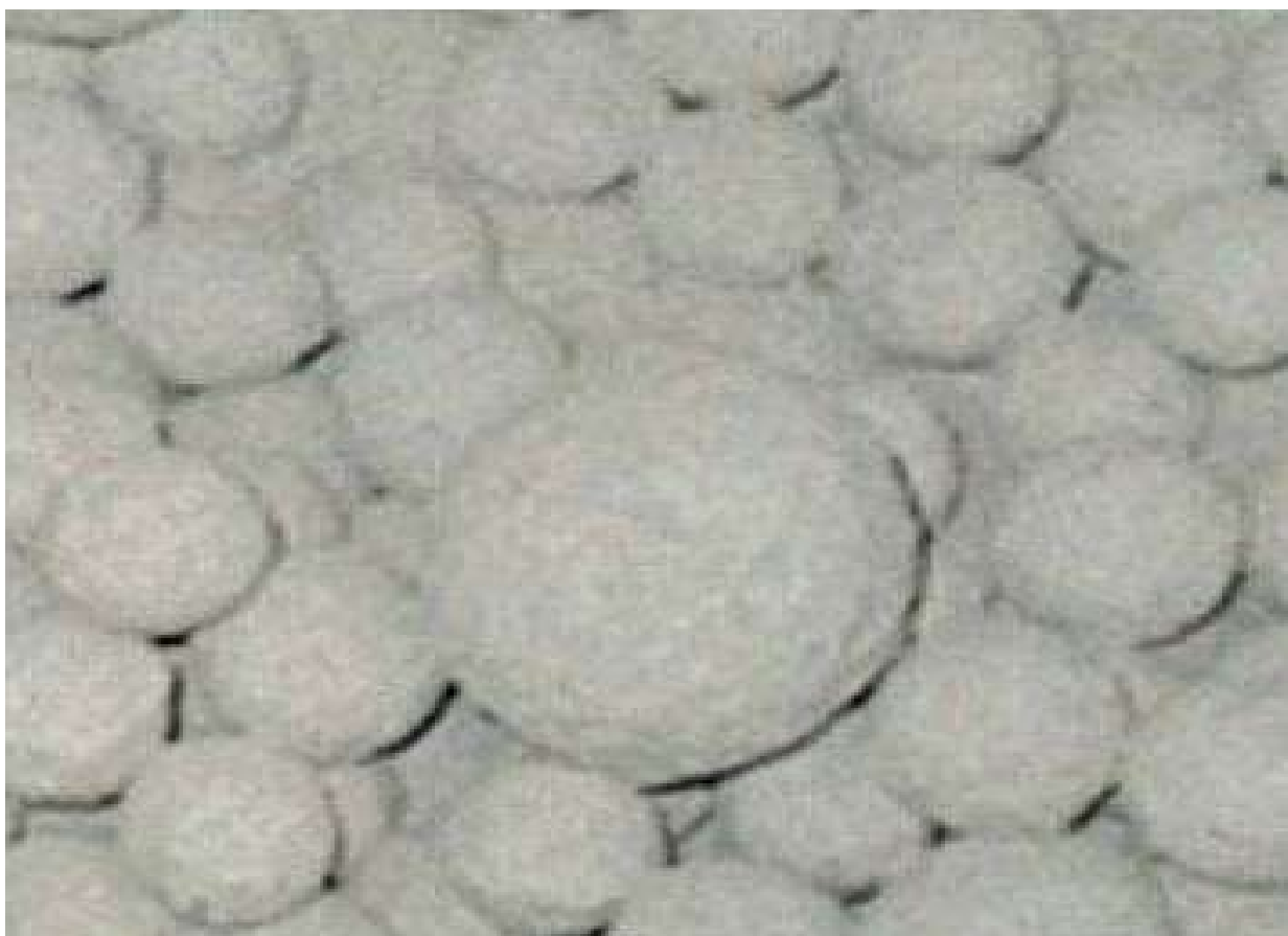
Ball mill grinding without grinding aids leading to coating on the balls and decreasing milling efficiency.
