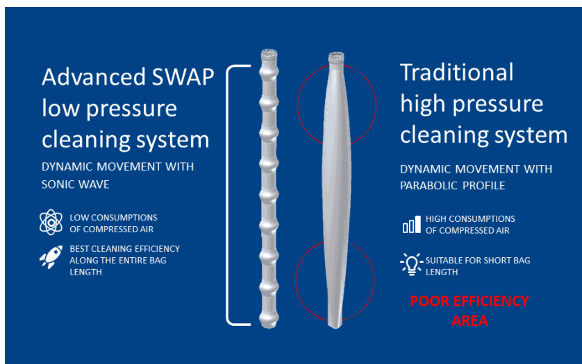
Figure1: The “cleaning efficiency” is a key parameter strictly connected to the level of emissions requested by our client. This parameter optimizes the bags arrangement* together with the type of filter media and the choice between of high or low compressed air pressure for cleaning system
