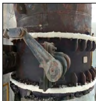
Fig 06: False Air Arresting by Arrest Master Range of Products.
