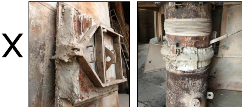
Fig 04: Conventional False Air arresting methods (By Sodium Silicate + Mortar/Raw Mill Powder, By Ceramic Blanket + Sodium Silicate)
