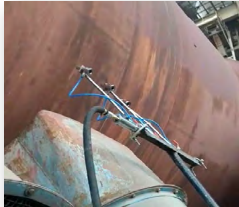
Fig 09: Kiln Shell cooling by Energy efficient device (Arrest Master ABS)
