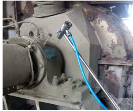
Fig 08: Bearing housing cooling by Energy efficient device (Arrest Master ABS)
