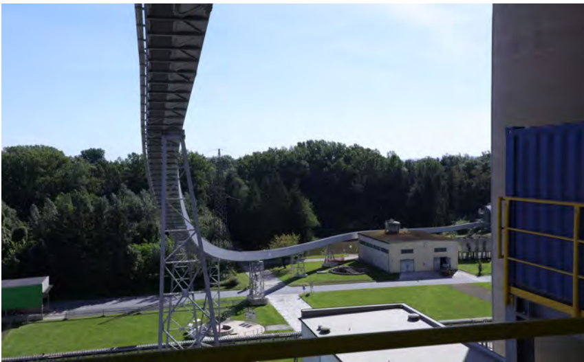
Figure 4: With the U-conveyor, tighter curve radii than with a troughed belt conveyor and higher mass flows than with a tube belt conveyor can be implemented.
