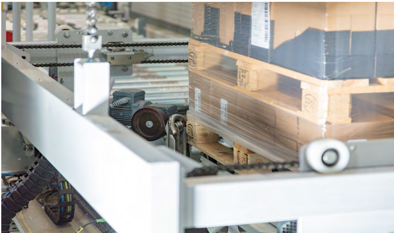
Photo 5: If the BEUMER stretch hood A packages the pallets for high-bay storage systems, the pallet base remains unwrapped, so that the forks of the fork-lift truck won't damage the film.
