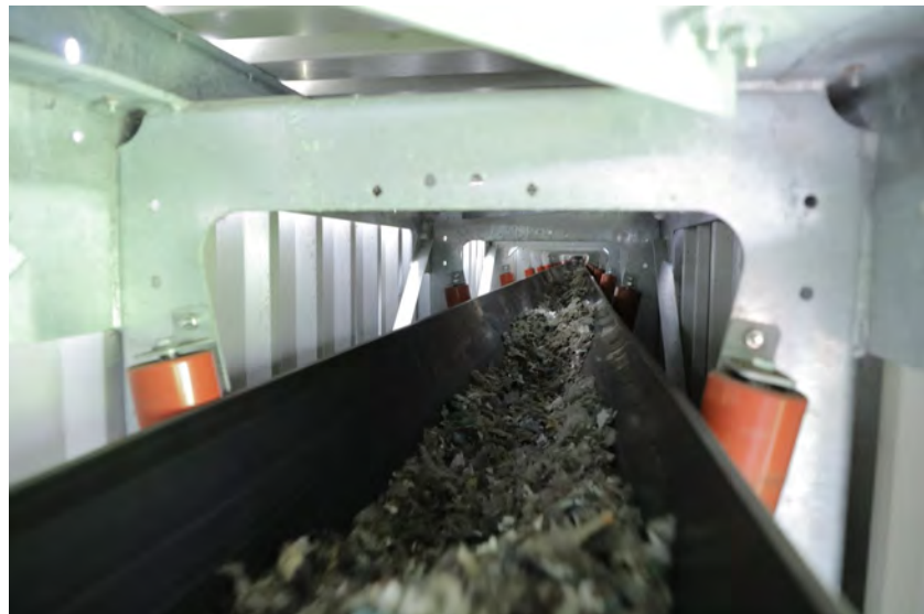
Figure 1: The U-conveyor: The idlers form the belt into a U.
