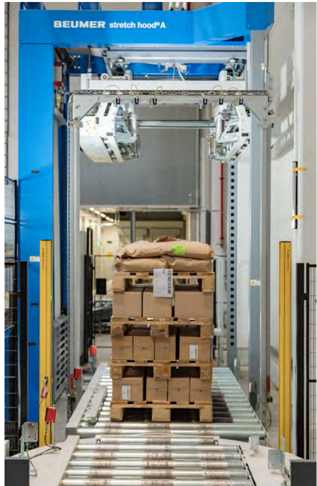
Photo 4: The pallets are packaged in short cycle times. The machine covers the products with a highly elastic stretch hood.
