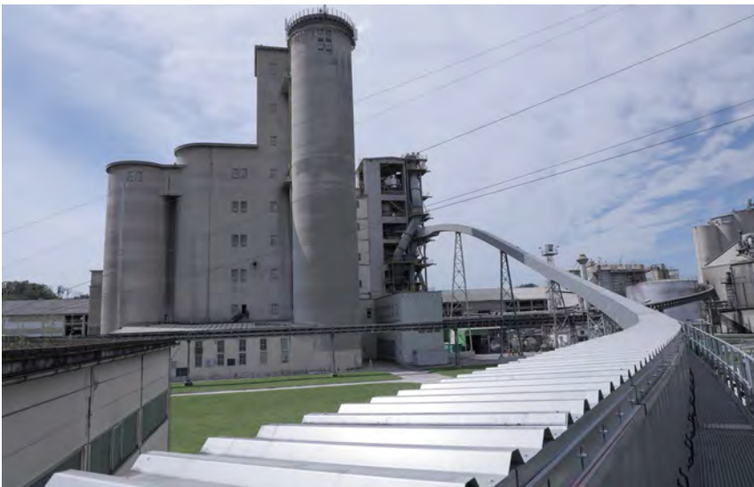
Figure 5: The conveyed material is protected against external influences such as wind, rain or snow - and the environment against potential material loss and possible emissions.
