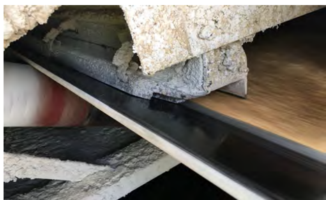
The clean belt edge shows the effect of the .AirScrape
