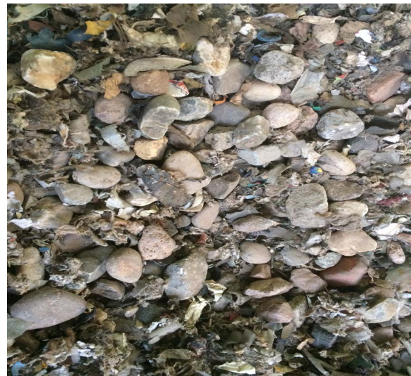
Figure 5: Typical heavy particles sorted out during the drying process by the included air sifting element; (a) – Case with basically metallic parts, hard plastics; (b) – Case with mainly mineral fractions, such as stones - (Image courtesy: DI MATTEO Group)
