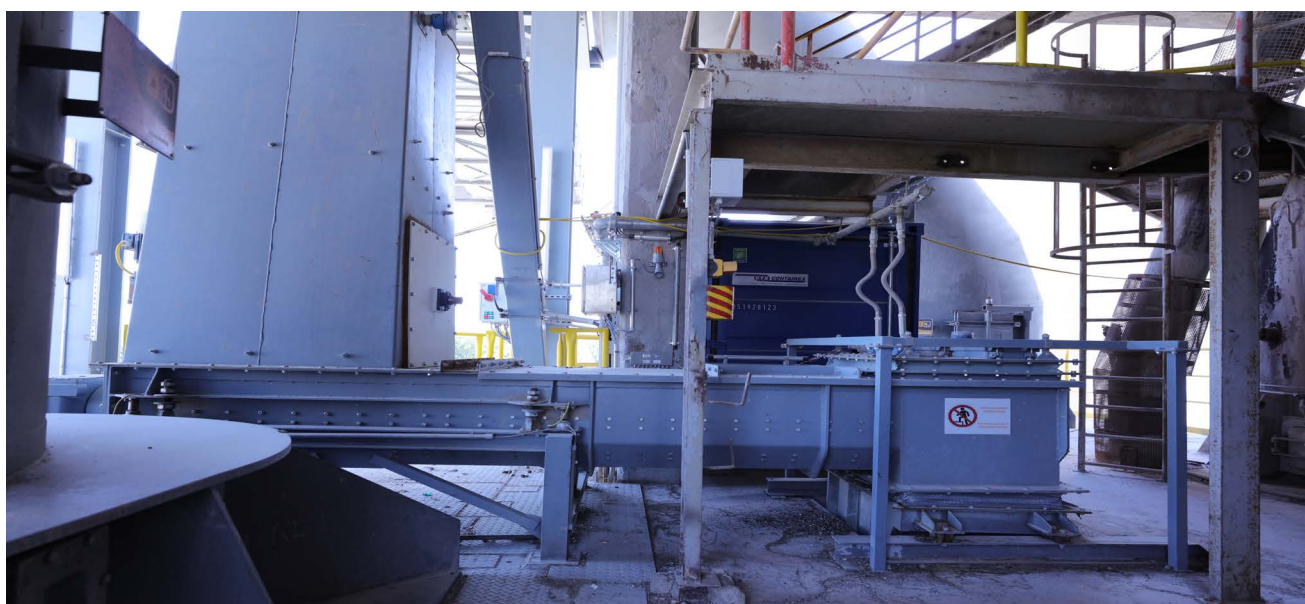
Picture 3: The double discharge screw conveyor of the BG OptiLock construction series: The airlock principle protects the material against the infiltrated air entering from outside.
