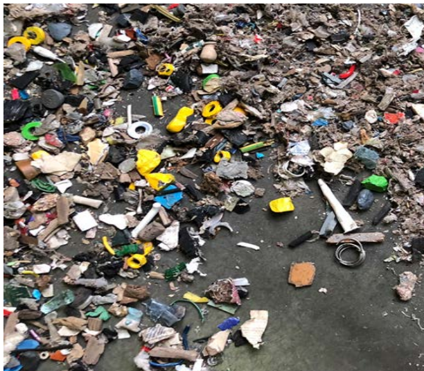
Figure 5: Typical heavy particles sorted out during the drying process by the included air sifting element; (a) – Case with basically metallic parts, hard plastics; (b) – Case with mainly mineral fractions, such as stones - (Image courtesy: DI MATTEO Group)
