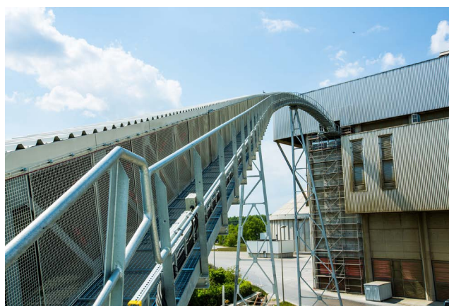
Picture 4: Pipe Conveyor: The enclosed system ensures an environmentally safe, dust-free and low-energy transport of the alternative fuels.
