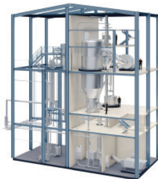
An essential part of pre-engineering is a layout plan of the main equipment - here with a fluid bed granulator as the heart of the plant
