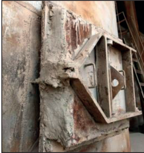
Fig 04: Conventional False Air arresting methods (By Sodium Silicate + Mortar/Raw Mill Powder, By Ceramic Blanket + Sodium Silicate)
