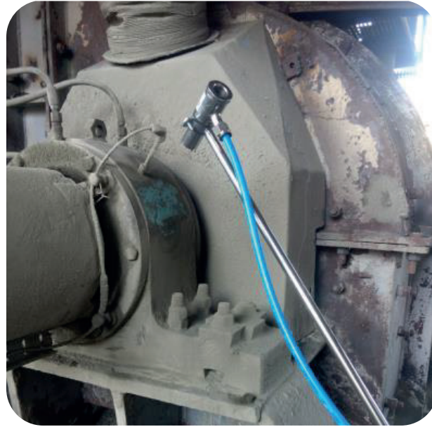
Bearing housing cooling by Energy efficient device (Arrest Master ABS) Input @ 6 Bar = 11 CFM, Output= 77 CFM, Atmospheric contribution= 66 CFM
