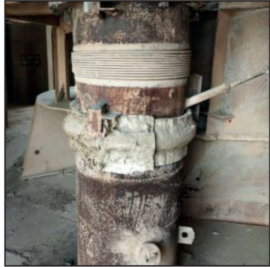
Fig 04: Conventional False Air arresting methods (By Sodium Silicate + Mortar/Raw Mill Powder, By Ceramic Blanket + Sodium Silicate)
