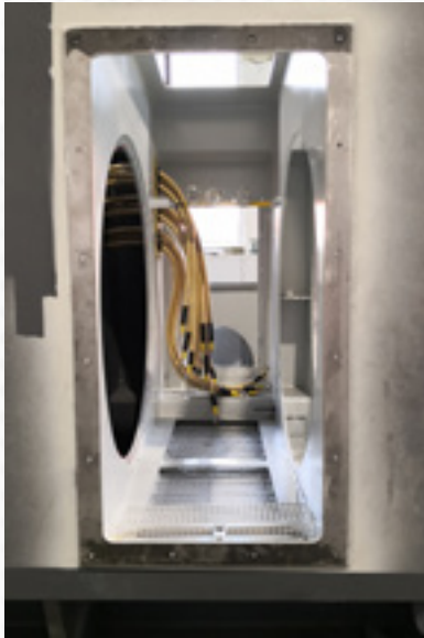
Images 4, 5: A roomy slip ring compartment, separated from the motor interior and with large service windows on both sides enables easy brush exchange in dusty environments (brush system shown before installation)
