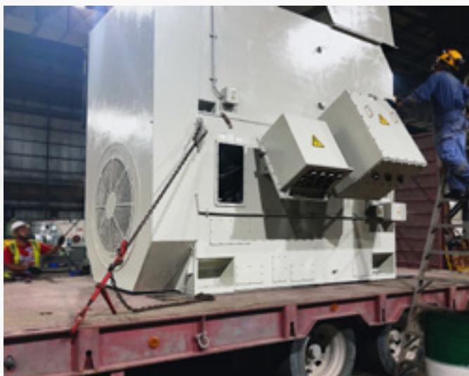
Image 1, 2: Menzel adopted the old motor's (left) tilted terminal boxes for the new motor (right) to enable plug-and-play installation in cramped conditions
