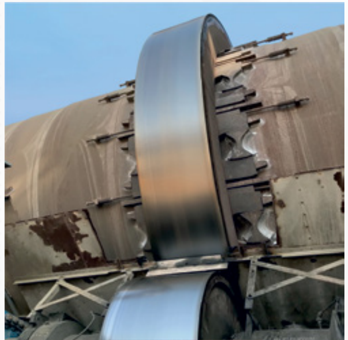
Figure 7: Insitu machined and grinded tyre and roller.
