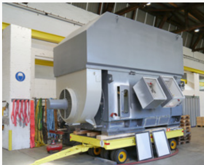
Image 1, 2: Menzel adopted the old motor's (left) tilted terminal boxes for the new motor (right) to enable plug-and-play installation in cramped conditions
