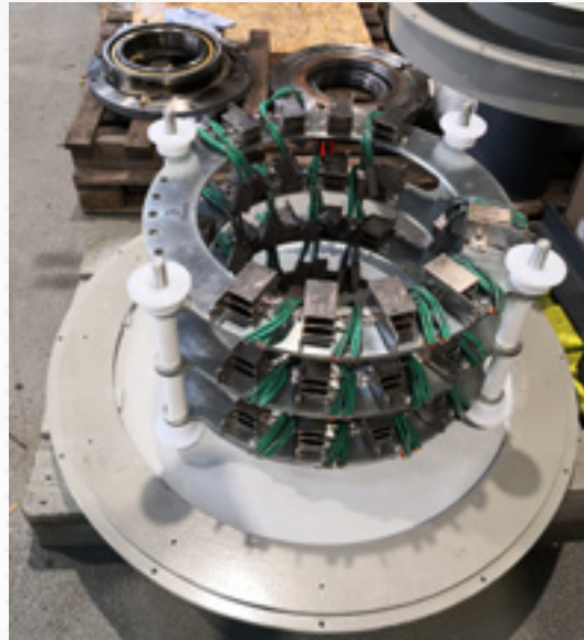
Images 4, 5: A roomy slip ring compartment, separated from the motor interior and with large service windows on both sides enables easy brush exchange in dusty environments (brush system shown before installation)
