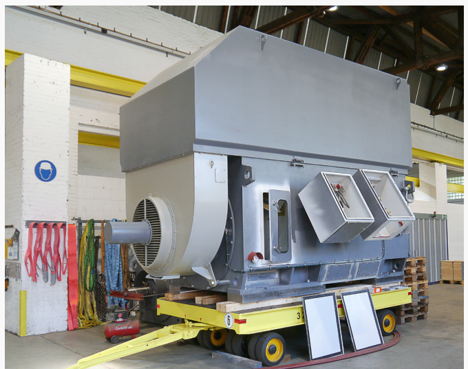
Image 1, 2: Menzel adopted the old motor's (left) tilted terminal boxes for the new motor (right) to enable plug-and-play installation in cramped conditions
