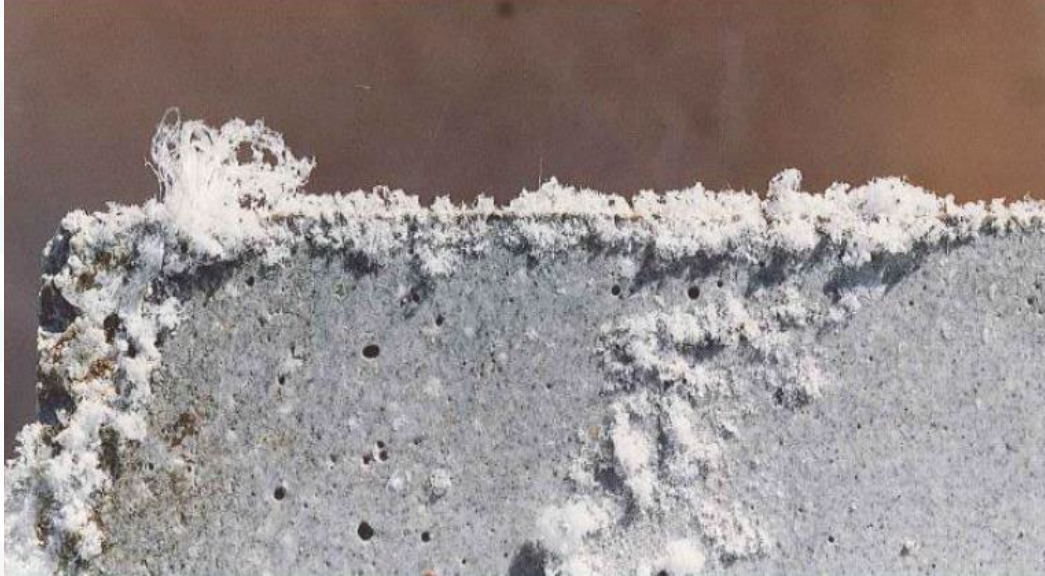
Fig-6, Carbonation of undried cast body.
