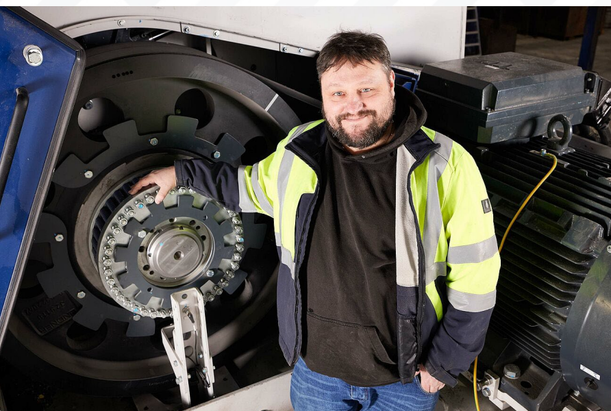
Daniel Vermeulen, Technical Operations Manager, in front of the Komet Series 3 belt drive incl. safety clutch and automatic belt tensioning system (ATB).
