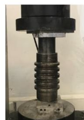
Figure 5. The Lump breaking force, that need to be applied to lumps after exposure at RH 100%, 50°C, within 24 hours.
