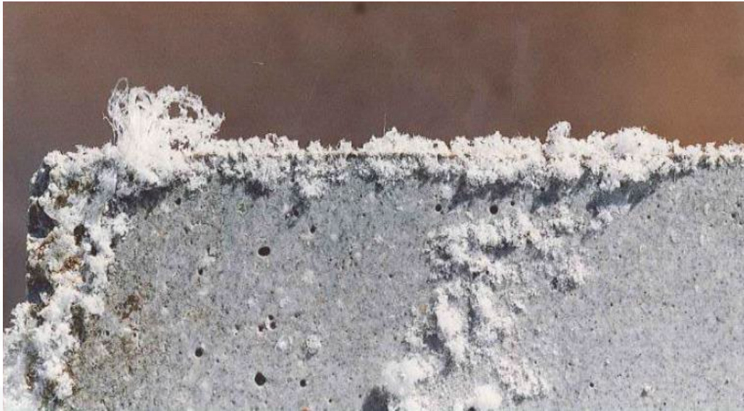
Fig-6, Carbonation of undried cast body.
