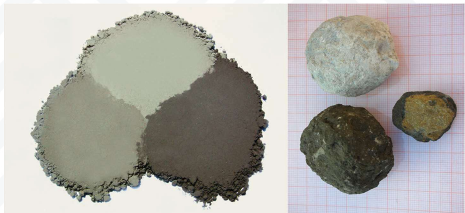
Fig. 1: Clinker burnt under normal, slightly reduced, and brown clinker caused by reductive burning conditions by incomplete burn-out
