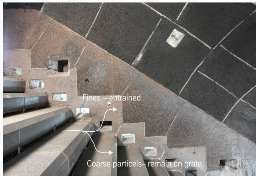
Separation of fine and coarse fraction of RDF during each air shock blast
