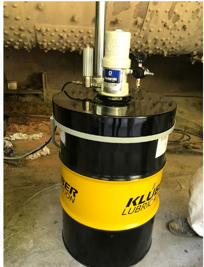
Graco Fire-Ball pump installation at VICAT, France.
